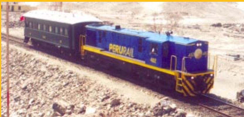
Constant inspection is the key and private cars “Ampato” and “Misti” are regularly taken out by management on inspection tours. In the photo, high nose 1200 HP ALCO/MLW No. 482 and inspection car “Ampato” roll through Quiswarani station (Km 135) on the Matarani - Arequipa section.
