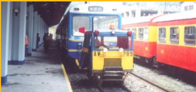
Another safety measure put into practice by management requires running protection vehicles in front of all passenger and freight trains on the standard gauge. On the narrow gauge, protection vehicles always run in front of the first train of the day. In the photo, “Autovía” No. gets ready to leave Aguas Calientes (new) station ahead of the first afternoon train back to Cusco’s San Pedro station.
